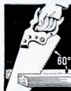
Proper angle for ripping
